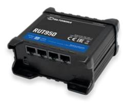
Rugged and durable professional 4G LTE Dual SIM cellular router with advanced WiFi, Ethernet and industrial grade networking functionality support. Quick to deploy, easy to manage and flexible for applications across most demanding market sectors.
