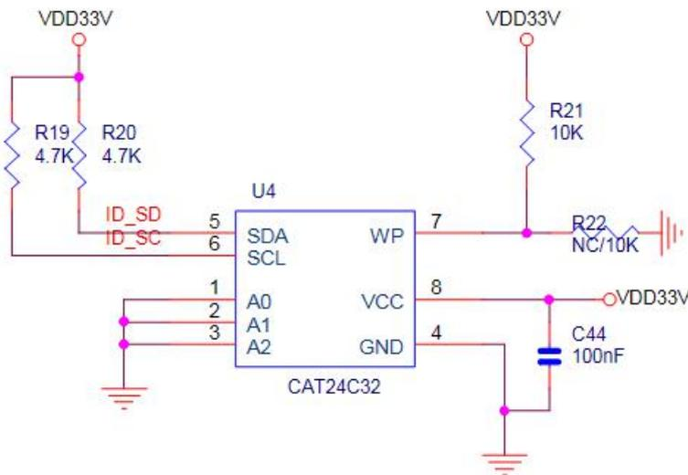
Pin 27 and 28 are always reserved for an ID EEPROM on the Raspberry Pi. Independently which card you use. It's useless for most application. If you want to use this function, you need to solder the IC, resistance and capacitance by yourself.
