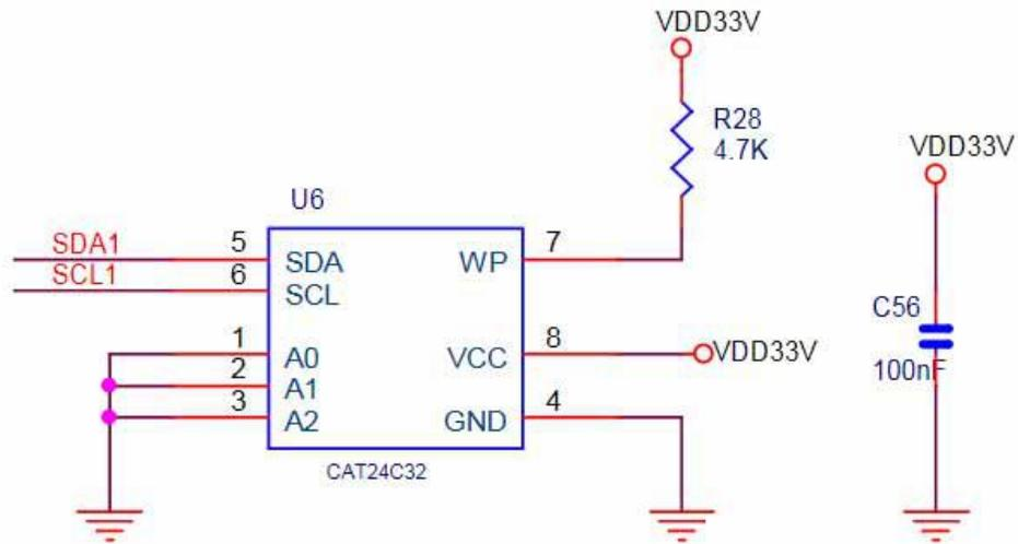
It connected to the same IIC port with AMP you need to solder the IC and Confirm IIC slave devices. If you a novice of Raspberry Pi, We really wouldn't advise do that.
