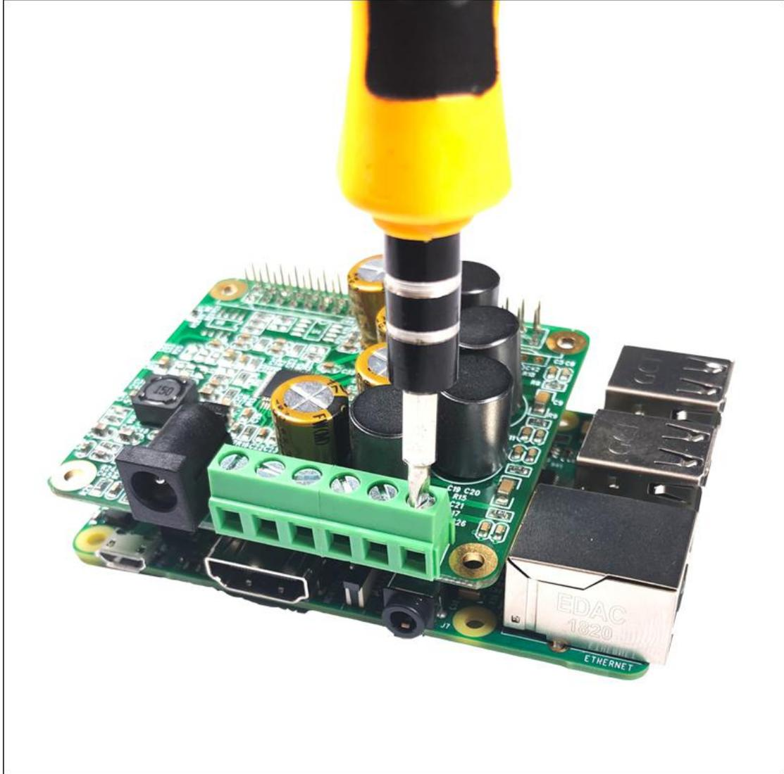
(2) And then plug the speaker cables into connector correctly and screw down. Please check the silk-screen on the back of the board.
