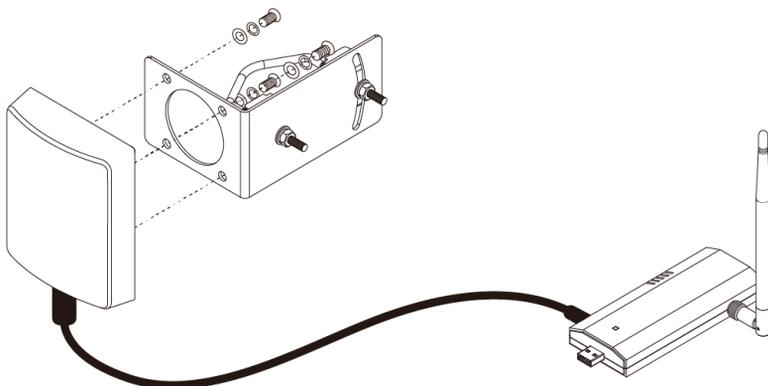
**APA-L2410A-P** 2.4 GHz 10 dBi directional antenna with pole mount
