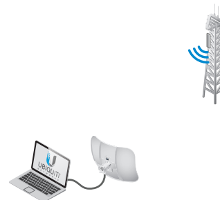
LiteBeam as a powerful wireless client.
