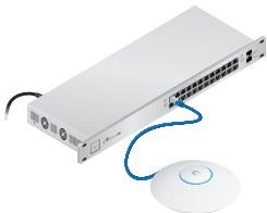
UniFi Switch with PoE Power Connection Diagram
