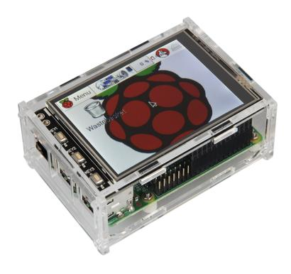
Build a small Tablet PC based on Raspberry in no time at all. This case was especially designed for the Raspberry (B+, 2B, 3B) and the 3.2" V2 Touch Display. It consists of high-quality, transparent acrylic.
