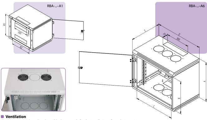
The RBA type A6\* has 6 break-out blanking panels for the installation of ventilation units RAx-CH-X2x-X1 or fans RAX-CH-X07-X9 (up to 3 in top and 3 in bottom part of the cabinet). The RBA cabinet provides with a possibility to install an equipment, which has never been cooled enough before. Such equipment could be only installed into free standing cabinets before.
