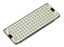
A sparkly 17x7 grid of snugly packed, individually controllable white LEDs to bling up your Raspberry Pi Pico, accompanied by a quartet of useful buttons.
