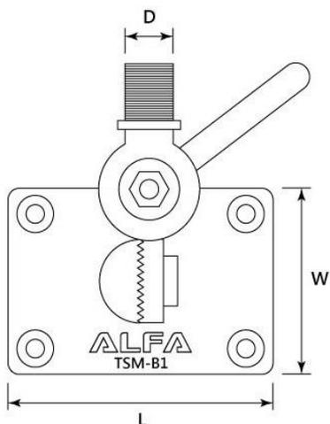
TSM-B1 is the stainless steel ratchet mount with versatile four-way design that adapts easily to deck or side mounting on slanted or level surface. The quick action handle makes raising and lowering the antenna easy and return the antenna to its correct, upright position. With TSM1, you could easy mount with ALFA Tube series device.
