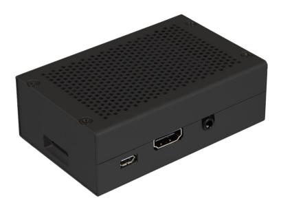
The housing can be assembled in a few easy steps and offers your Raspberry sufficient protection due to its sturdy construction. The Raspberry is also ventilated through the openings on the top of the housing. All connections are easily accessible, even the SD card slot on the underside of the Raspberry can still be used.
